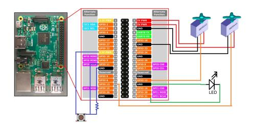
Figure 3.2: Pin mapping of the Raspberry pi
