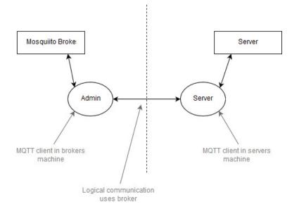
Figure 3.10: Server broker architecture
